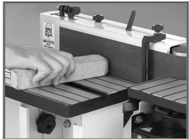
Figure 27. Cleaning the sanding belt with PRO STICK®.
